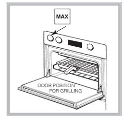
**Step 1** Place the oven shelf in the correct position (see Grilling Guide). Locate the grill pan on the oven shelf, centrally under the grill element. Leave the door fully open.
