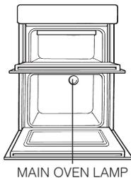
**Warning: To avoid electric shocks - please ensure that the electricity supply to the appliance is switched off and the appliance is fully cold, before removing the lamp lens.**
