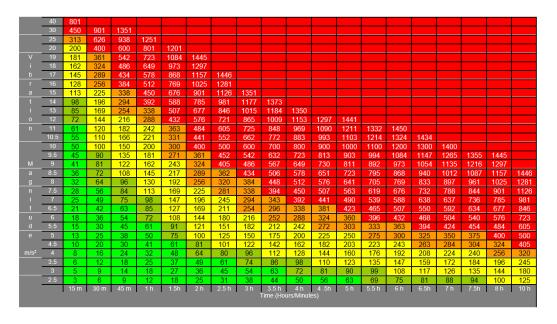
Use the Ready Reckoner to manage and plan your tool usage at the start of the day to ensure that your Exposure Limit Value will not be exceeded. It is too late to identify that you are exceeding the 400 points Exposure Limit Value before the end of your working day.
